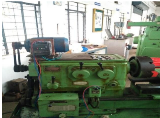
Fig 3. Experimental setup of stepless power transmission to the lathe
